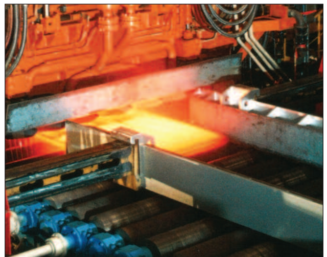
Steel mills. Couplings fitted to table roller drives on rolling mills and furnace discharge tables.
