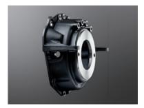
For connecting hydraulic pumps to the diesel engine KTR supplies mounting flanges according to SAE connection dimensions sizes SAE 6 to SAE 1. These flanges are made of steel and ENGJL-250 (GG25) for hydraulic pumps with flange connections according to SAE-A, -B, -C, -D and -E as types with 2 and 4 holes.
